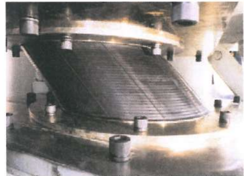
SSI® Earthquake Simulation: Combined Shear & Vertical Loads
